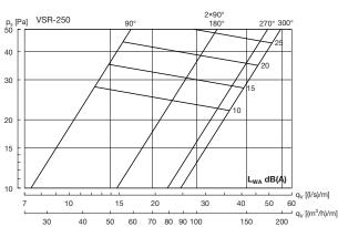
The sound levels from the nozzles apply for duct length 1 m.
