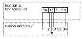
Additional connected dampers (not connected in groups) are connected in the same way in terminal 20-47.
