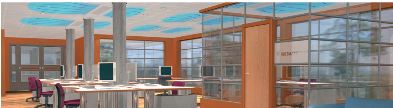
Picture 6. A separate office is to be fitted into the room. If the climate is to be optimal, the air quantity and air volume need to be adjusted for the Premium beam that will be built into the new room.
