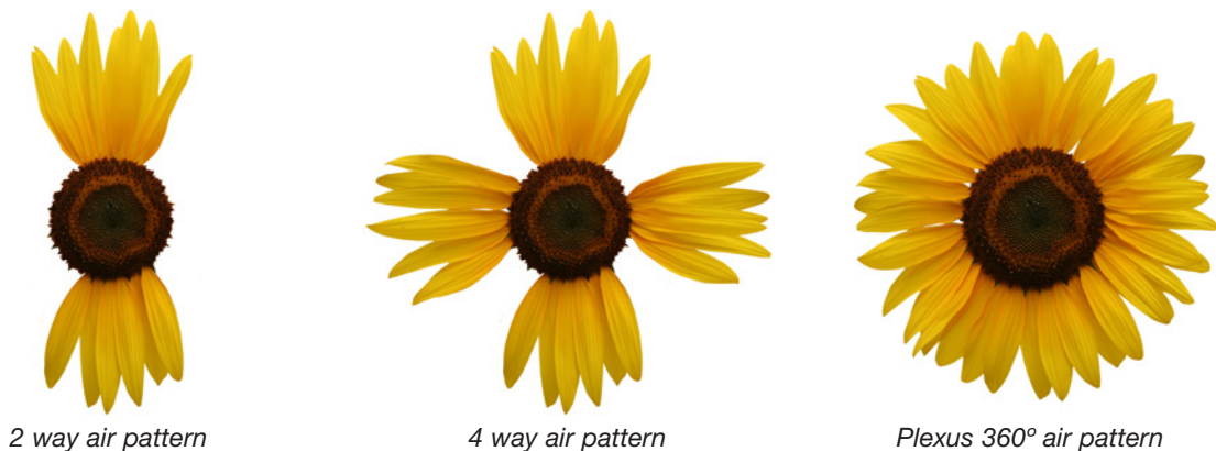
Picture 1. Plexus integrates both cooling and heating functions from the climate beams together with the supply air terminals technique. Unique for the Plexus is that the air is supplied in a 360° air pattern instead of a traditional 4 way pattern. This feature allows approximately 30% shorter air throws.
